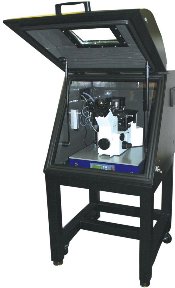
AEK-2002 in use with an AFM, confocal microscope, and TS active isolation system.
